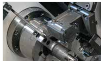
Chuck Air Blow (Upper Chuck)
